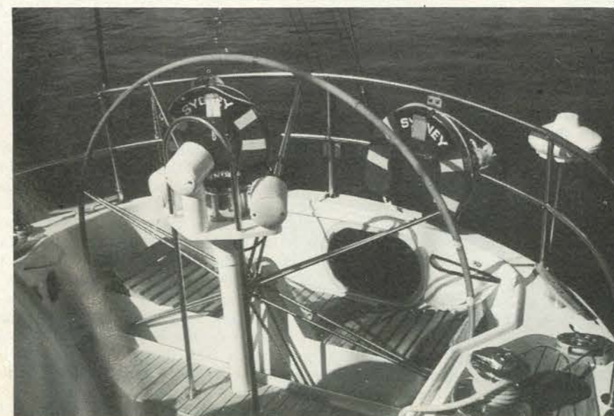
The large stainless steel wheel, with a leather cover, is partially sunken into the cockpit floor.
