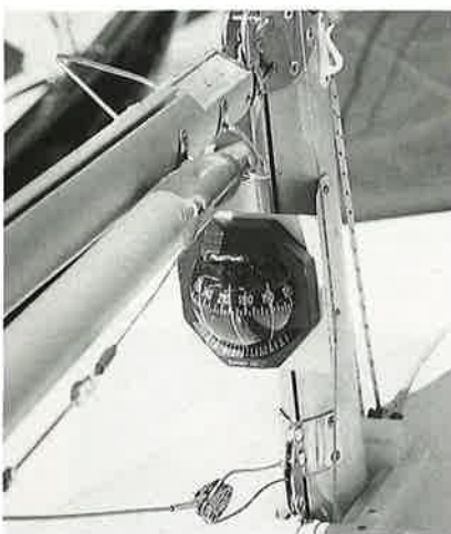
MAST-mounted Plastimo compass is easily read from all angles, while, BELOW, the set-up for fine tuning of the jib — all within easy reach of fo'ard hand.
