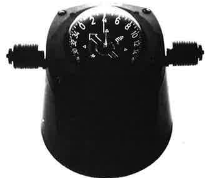
SILVA 105 PBEC-S For ferrocement and steel boats. Pedestal mounting with B, C coefficients, corrector for D coefficient, and heeling corrector magnets. 12v light system. 175mm diam. base.
