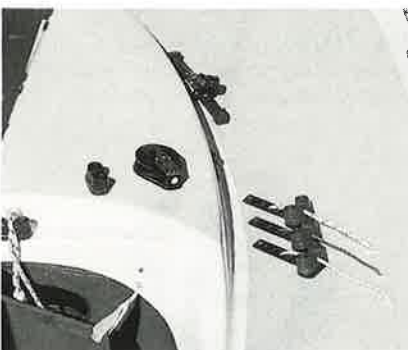
MAST-mounted Plastimo compass is easily read from all angles, while, BELOW, the set-up for fine tuning of the jib — all within easy reach of fo'ard hand.
