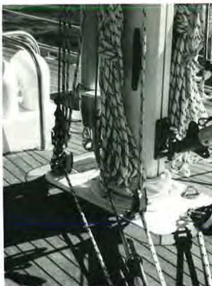
DECK area around the mast of the Wayworld 45 is free of winches, with halyards, topping lift and son running aft through rope clutches to winches located near cockpit. (Pic — Rob Williams)
