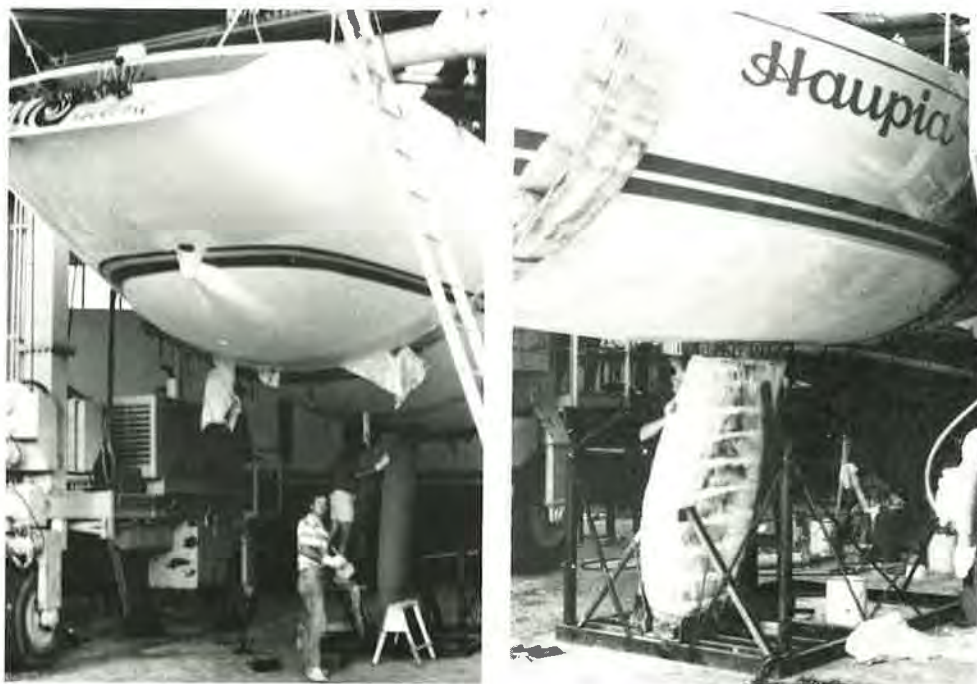
Cyclone and Haupia are fitted with their new keels
