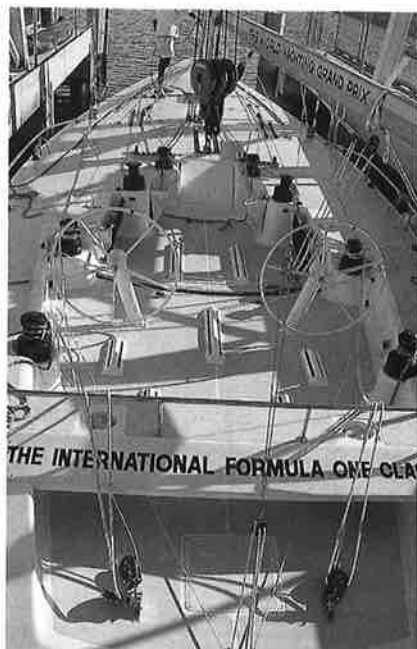
DROPPING the huge spinnaker of the Formula One 52 during test sail off Fremantle. Below, the deck layout of the Formula One, showing twin wheels, good crew working areas. (Pics — John Roberson).
