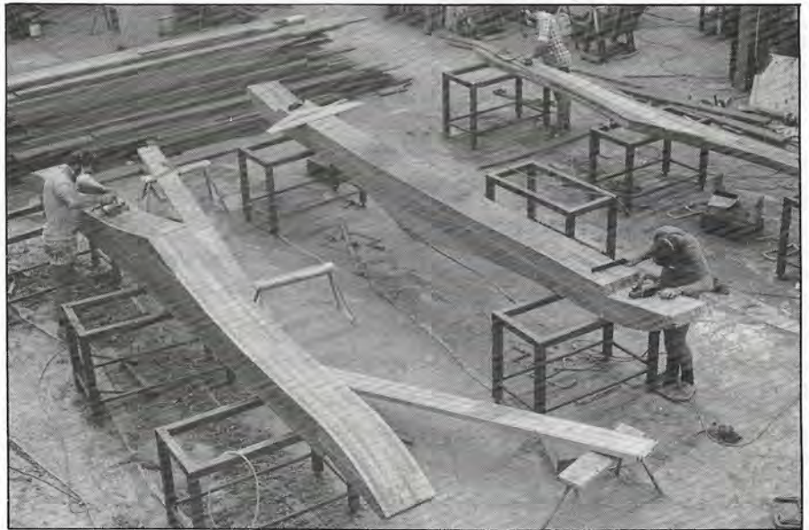
BOATBUILDER Steve Ward, who built Alan Bond's famous 12-metres, including America's Cup winner AUSTRALIA II, has transferred his talents to constructing the wooden-hulled replica of ENDEAVOUR. LEFT: shows Ward with prefabricated jarrah frames for the 106-foot ENDEAVOUR. BELOW: shipwrights prepare the floors for the ENDEAVOUR which will be assembled on Fremantle foreshore. (Peter Campbell pics).
