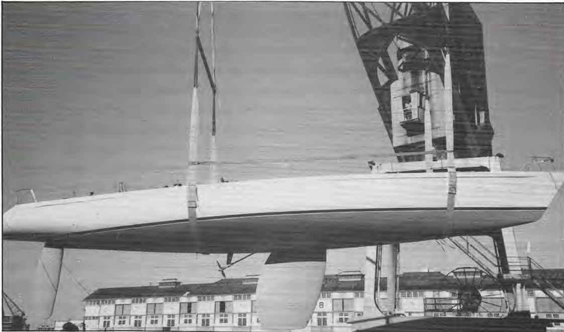
WINDWARD PASSAGE II is lifted into the water, revealing long shallow body and deep keel and rudder.
