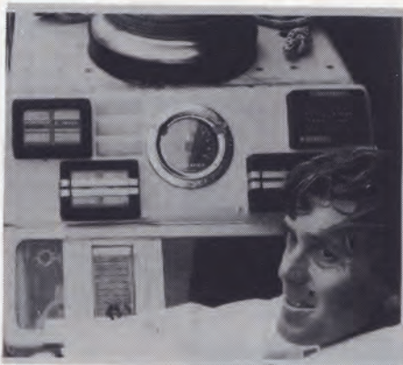
Halsey Herreshoff, navigator of Freedom, is pictured above in front of the console which contained the H-P computer (inside the panel at the right). Wind and current readouts are at the top, and an HP-41C hand-held calculator, for mid-race computation of statistics, is at mid left. Picture at the left shows where console was located.
