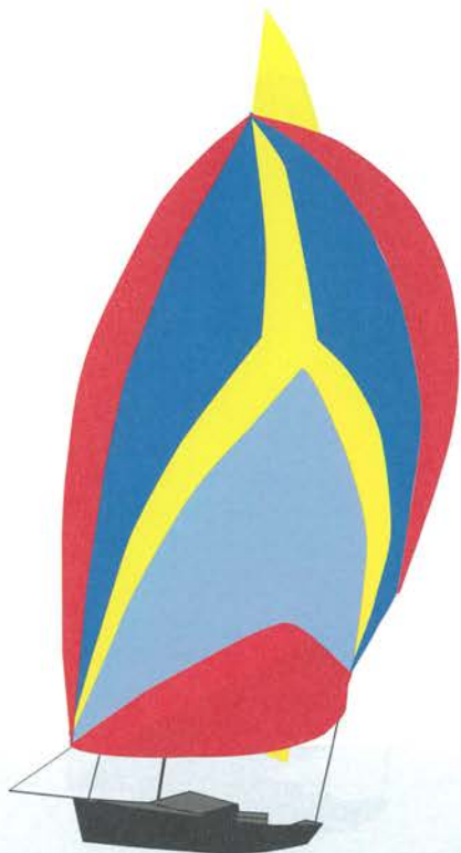
FIGURE 4: IF THE SAIL FALLS TO LEEWARD WHEN THE TACK LINE IS EASED THEN KEEP THE TACK LINE SNUGGED DOWN TO THE SPRIT
