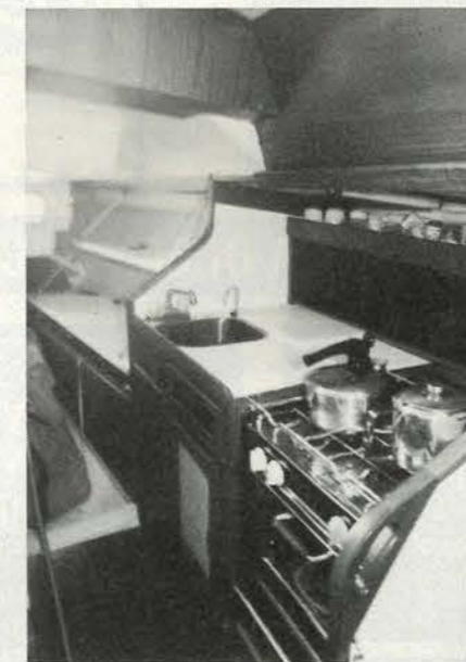
On the port side of the companionway is the galley. A gas stove and oven is fitted as is hot and cold water.
