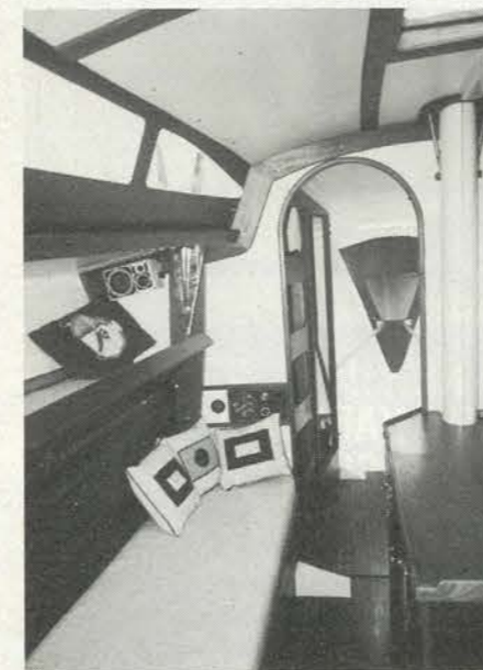
The main cabin has two berths either side. Both are cushioned in a nice bone-coloured material over plastic. The lower bunks have lee cloths while the uppers have folding lee boards, doubling as a back rest when lowered.
