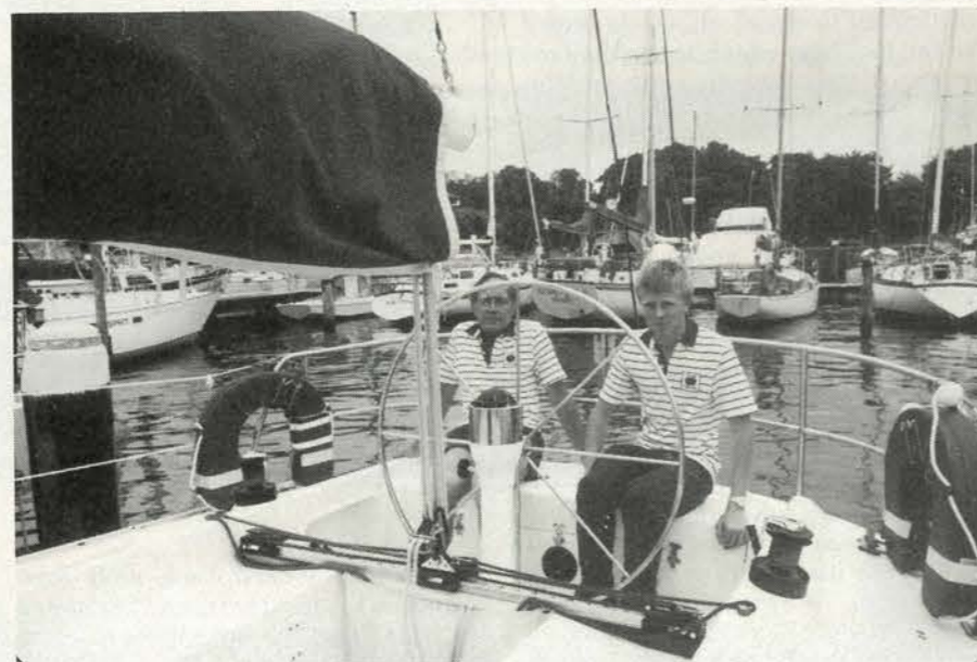
The cockpit is well laid out with storage lockers to the rear of the helmsman. The main is sheeted right across the cockpit immediately in front of the pedestal. Coamings are very nicely shaped to support crewmen when the boat heels. Pictured are skipper Bill Sweetapple and his son, Jamie.
