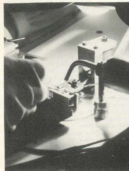
AWA technology at work; ultrasonic cold welding aluminium wire from an integrated circuit chip to its encapsulating package.
