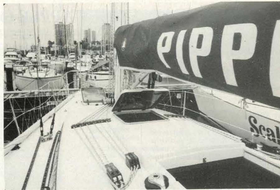
Tidy deck layout with jammers mounted in front of Barlow self-tailing winches. Pippin has rod rigging, hydraulic vang and backstay.
