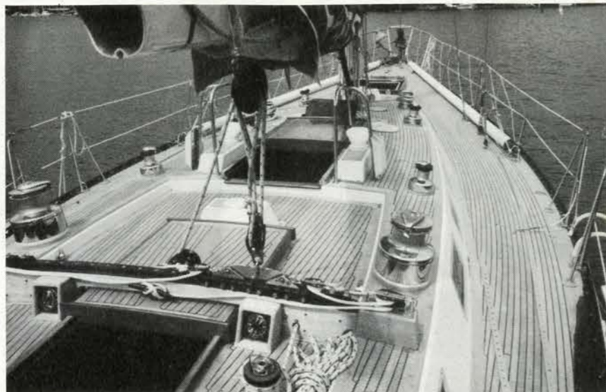
Centrefold has a teak laid deck, with 14 self-tailing winches.
