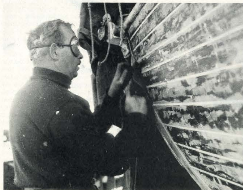
Don Mickleborough hard at work splining Southerly's hull in 1961.
