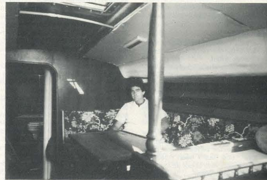
Poste Restante features a full-size chart table to starboard at the foot of the companionway; to starboard is an eight seater U-shaped lounge/dinette around a table which collapses to form a double bunk and to port a small seat. In front of the main bulkhead is a sail storage area to starboard and cupboard space to port, and forward again is a large separate toilet.
