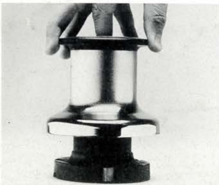
2. The winch top and drum dismantle from the base in one easy action.
