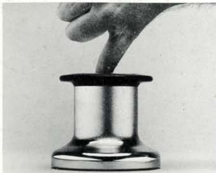
1. Push your finger down the throat of the Barlow winch and press the snap lock release button.*
