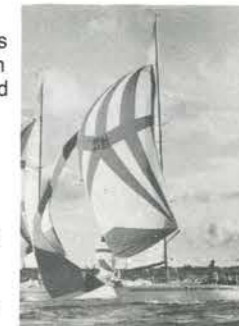
THE ROPERUNNER — KZ 4499 LOA 12.1 m; LWL 9.1 m; Beam 4 m; Draft 2.1 m
