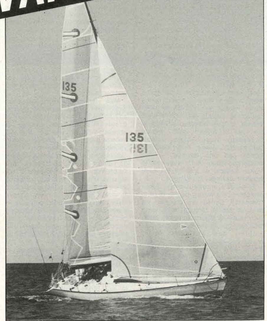
New Queensland Farr 40, The Gambler sports twin-ply Mylar headsail and composite Kevlar/Mylar main. Mike Power pic.
