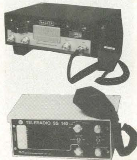
Marine radios have crystal-locked frequencies and are relatively easy to operate.
