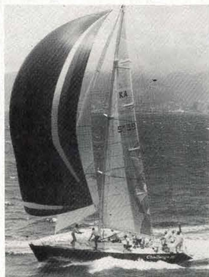
CHALLENGE III — KA SM39 LOA 42'7" / 13.0 m IOR 33.1 Construction: Carbon/foam/Kevlar Date: 1984 Owner/Skipper: Lou Abrahams Designer: Frers AUSTRALIA
