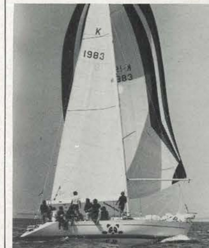
PANDA — K 1985 LOA 42'4" / 12.9 m IOR 30.5 Construction: Epoxy composite Date: 1985 Owner/Skipper: Peter Whipp Designer: Briand
