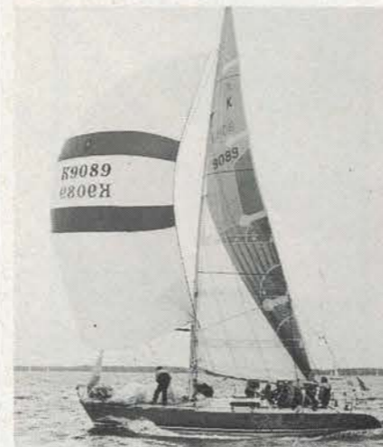
CIFRALINE 3 — K 9089 LOA 40' / 12.2 m IOR 30.5 Construction: S-Glass/foam sandwich Date: 1984 Owner/Skipper: Chris Griffin Designer: Andrieu
