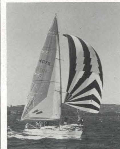
PALADIN — 4070 LOA 40' / 12.2 m IOR 30.5 Construction: Exotic core Date: 1985 Owner/Skipper: Colin Franklin Designer: Farr NEW SOUTH WALES
