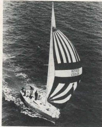
EXADOR — KZ 323 LOA 40' / 12.2 m IOR 30.2 Construction: Kevlar/S-Glass/Divinycell Date: 1983 Owner/Skipper: Michael Clark Designer: Clark NEW ZEALAND 'A'
