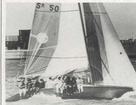
JOINT VENTURE — SM 50 LOA 40' / 12.2 m IOR 30.5 Construction: Kevlar/carbon fibre/Divinycell Date: 1985 Owner/Skipper: Ron Elliott Designer: Frers
