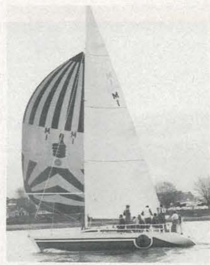
THUMBS UP — M 1 LOA 39' / 11.9 m IOR 30.5 Construction: Kevlar/GRP/Timber Date: 1985 Owner/Skipper: Tony Roland Designer: Adams/Radford
