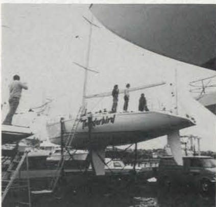
THUNDERBIRD — KZ 5855 LOA 43' / 13.1 m IOR 33.3 Construction: Kevlar/Divinycell Date: 1985 Owner/Skipper: Don St Clair Brown Designer: Farr NEW ZEALAND 'B'
