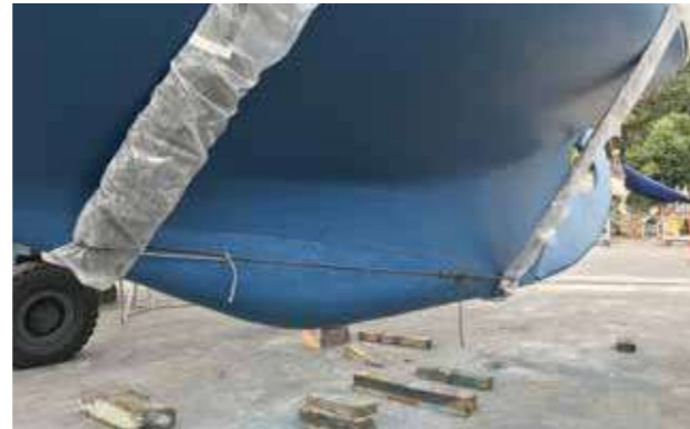
Sling time to access and antifoul under keel areas
