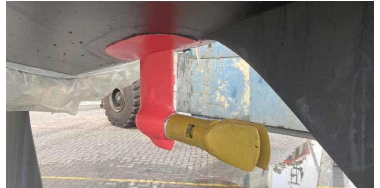
Non copper antifoulant on alloy sail drive and propspeed silicone on propellor
