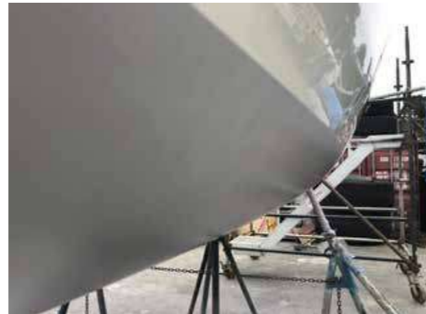
Hard antifoulant V.C offshore applied by airless spray
