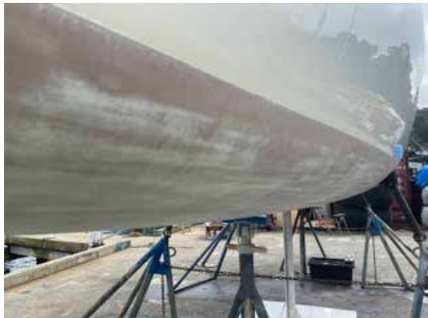
Wet sand hull preparation
